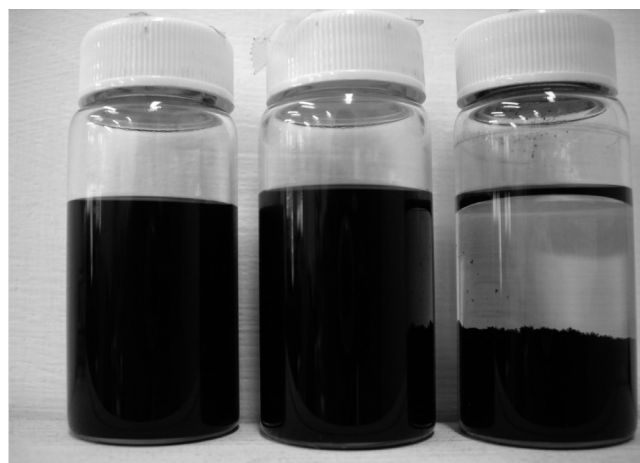
FIGURE 4. Photograph showing the dispersion of graphene, F-graphene/MA-POA2000, and D-graphene/MA-POA2000 in THF (from right to left). The photograph was taken after storage for 2 months with a concentration of 0.25 \text{mg mL}^{-1} .
